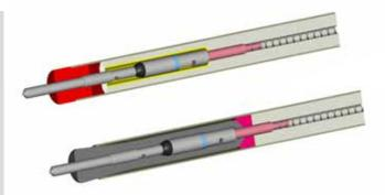
Tubular element with mounted thermal fuse.
